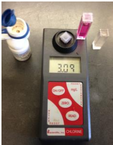
Chlorine testing in Water
