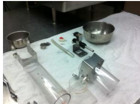
Swab method to culture ice machine components
