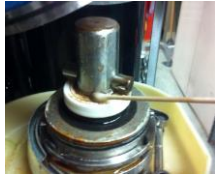
Swab method to culture ice machine components
